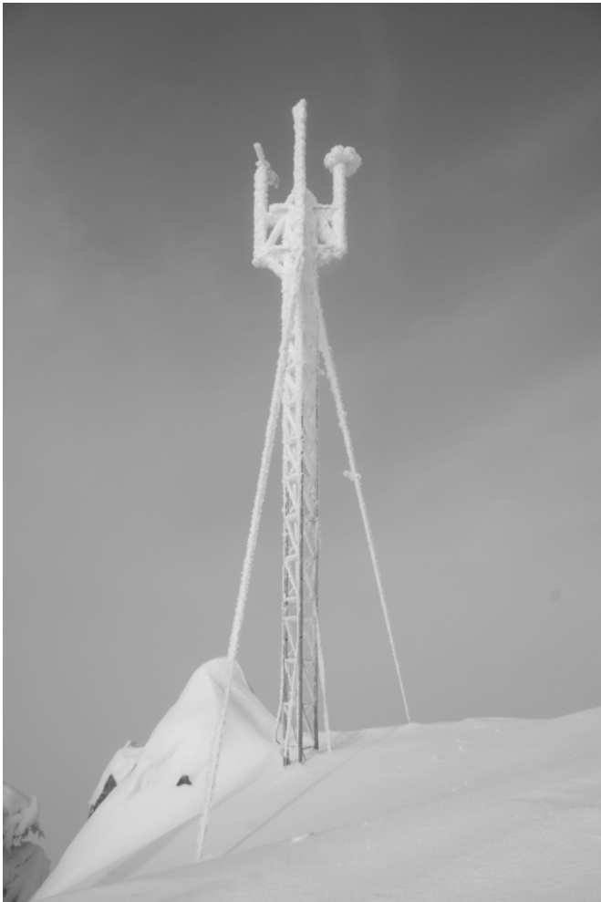
Figure D.5 A weather station coated in rime ice (photograph by John Stimberis).
